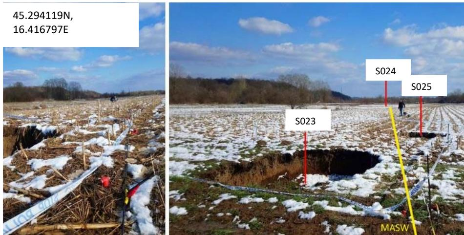
**Figure 10.8** MASW spread adjacent to three small sinkholes S023, S024, S025 in Borojevići.
