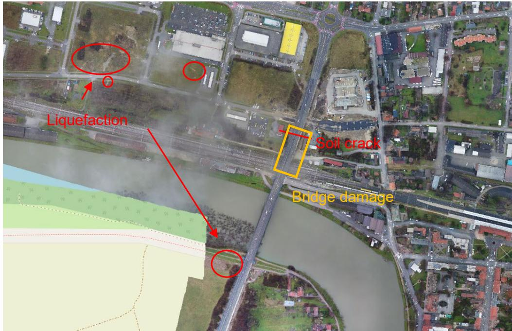
**Figure 9.19** Aerial view of the area with “Most Gromova” bridge after the earthquake.
