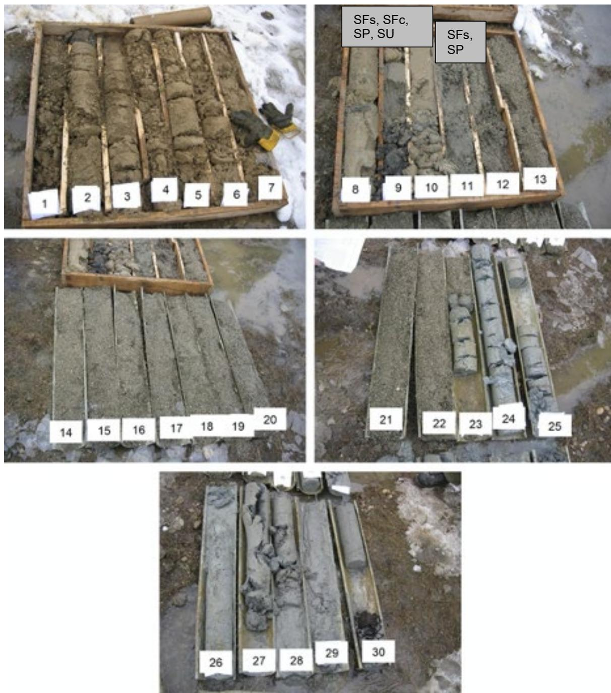
**Figure 3.6** Soil cores taken from the area near the thermal powerplant in Sisak, Čret (45.4538, 16.4145) (Marić, 2005).
