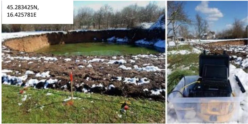
**Figure 10.7** MASW spread near the largest sinkhole S001 in Mečenčani.
