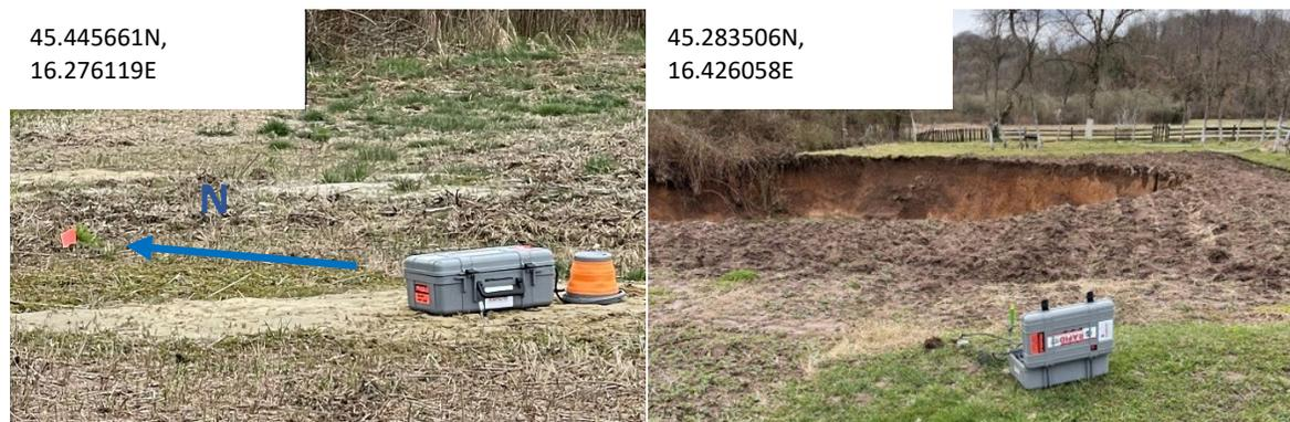
**Figure 10.1** Nanometrics setup, with a seismometer aligned to the North.
